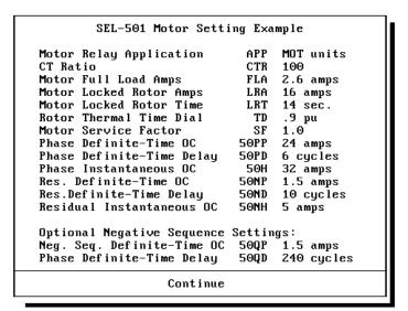
Figure 14: Motor Relay Settings
