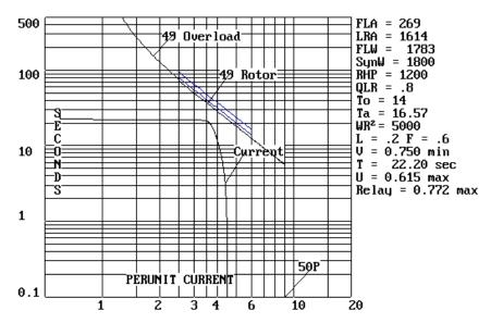
Figure 13: Log Plot of Current and SEL-501 Characteristic
