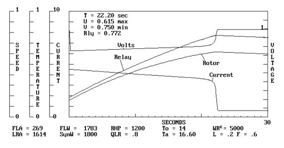
Figure 12: Plot of Motor Voltage, Current, and Rotor Hot Spot Temperature
