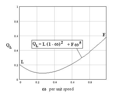
Figure 5: Contour of Load Torque
