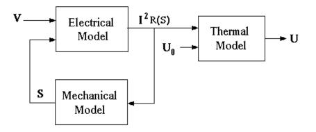
Figure 1: Motor Analysis Block Diagram
