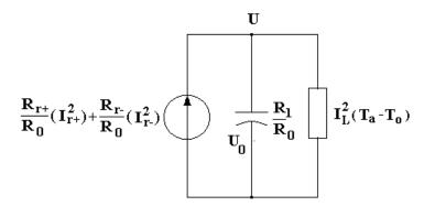
Figure 10: Motor Thermal Model
