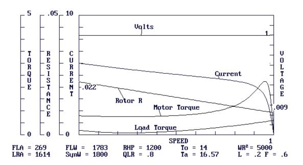
Figure 4: Current and Torque Versus Slip
