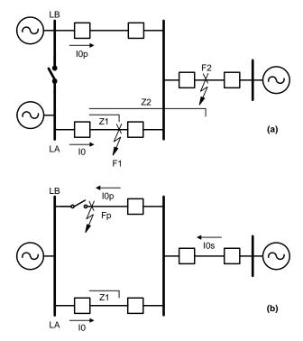
Fig. 13. Parallel Lines With a Single Common Bus
