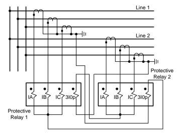
Fig. 16. Parallel Line 3I0 Current Circuits Cabling
