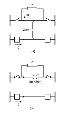
Fig. 5. Simple Ways to Visualize the Zero-Sequence Mutual Coupling in Parallel Lines
