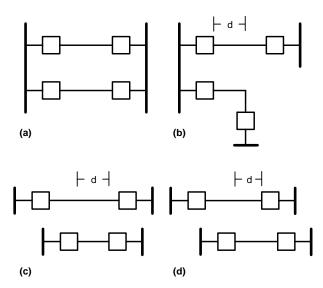
Fig. 1. Possible Configurations of Parallel Lines in Power Systems
