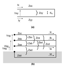
Fig. 2. (a) Two-Conductor Model (b) Three-Phase System With "Equivalent" Ground Conductor
