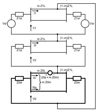
Fig. 6. Phase-to-Ground Fault in One of Two Parallel Lines With Zero-Sequence Mutual coupling
