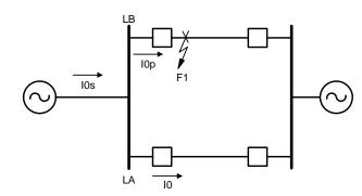
Fig. 15. Strong Source, Parallel Line Ground Fault Effect on the Healthy Line-Relay
