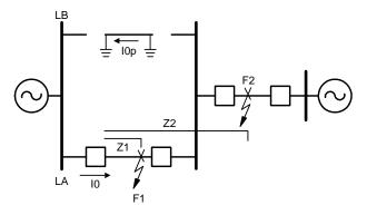
Fig. 12. One Line Grounded
