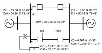
Fig. 14. 230kV Parallel Line Example
