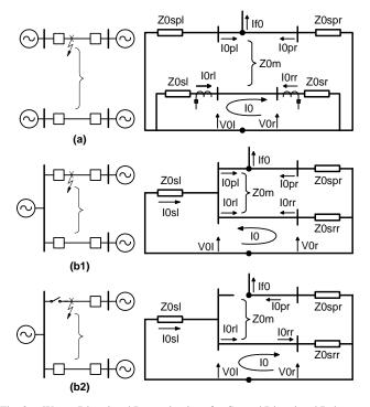
Fig. 8. Wrong Directional Determinations for Ground Directional Relays
