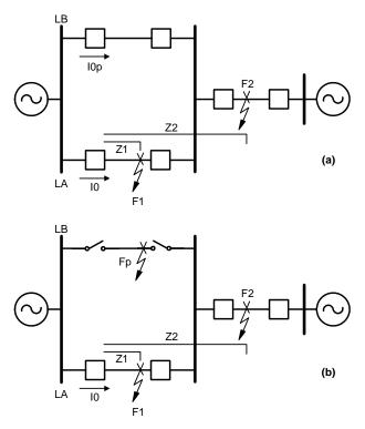
Fig. 10. Underreaching and Overreaching Zones in a Parallel Line Application
