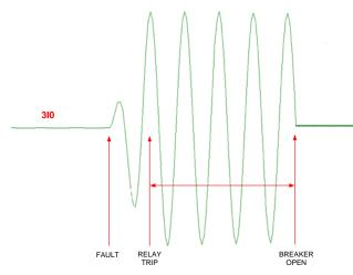
Fig. 17. Filtered 3I0 and Fault Clearing Sequence
