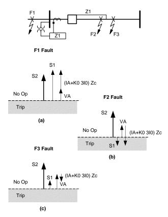
Fig. 9. Distance Relay Operation
