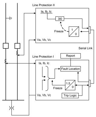
Fig. 18. Fault Location 3I0p Compensation With a Serial Link
