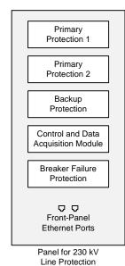
Fig. 12. Ethernet connection points on the front panel
