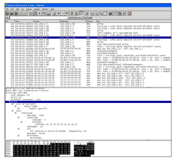
Fig. 6. Control operation sniffering through Ethernet analyzer
