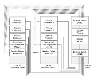
Fig. 10. System network architecture based on SICLE specification
