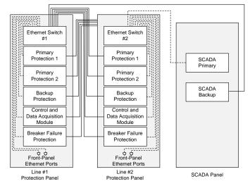
Fig. 11. System network architecture based on substation automation system specification
