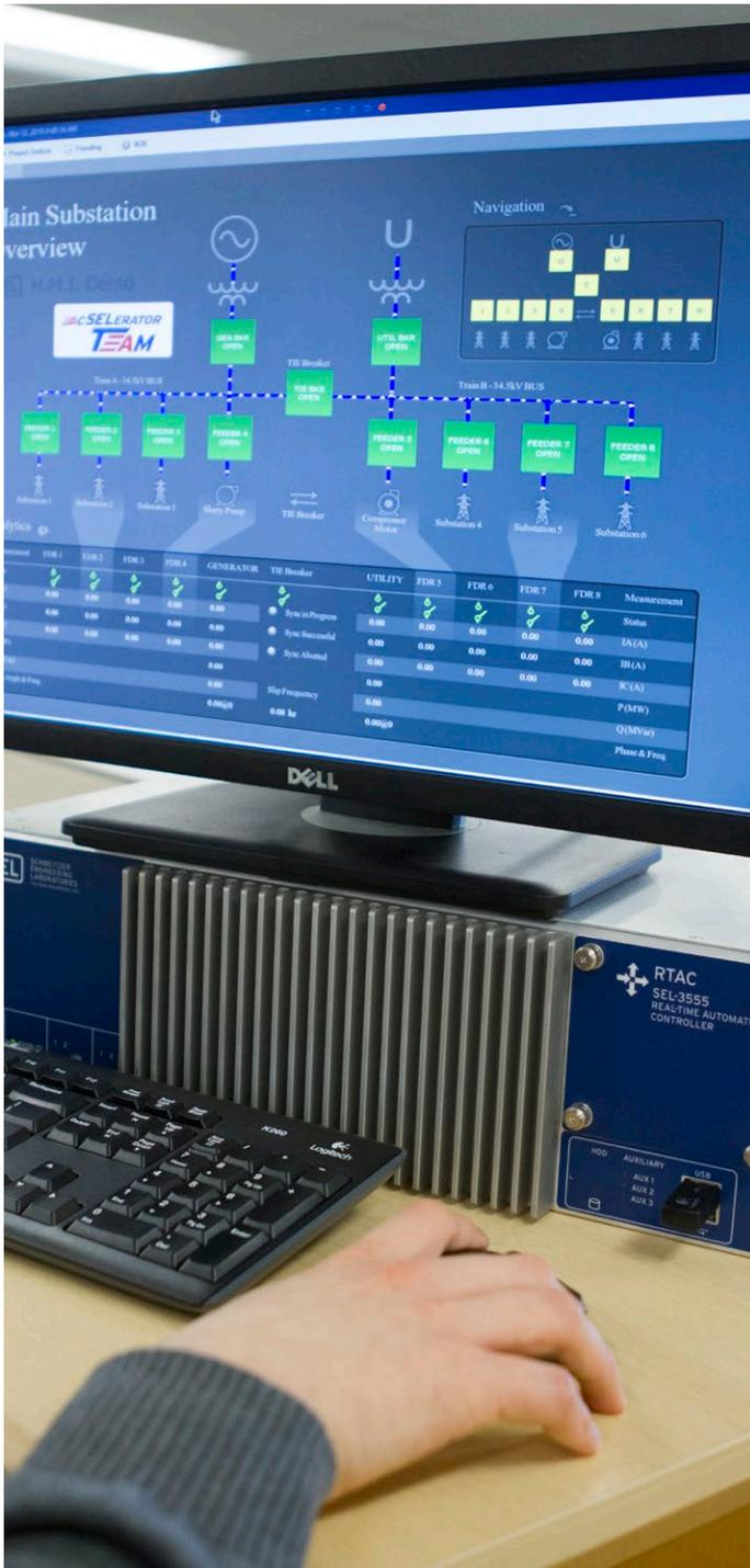
With advanced HTML5 technology, the RTAC HMI makes it easy to visualize data and create custom diagrams to monitor and control your system. The HMI allows authenticated access for multiple users and locations and is also viewable from a remote web browser. The video output port on the SEL-3555 RTAC connects directly to a monitor, allowing you to quickly and locally view HMI and SOE data without the need for an additional computer.
