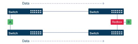
PRP provides redundancy via a duplicate network. PRP sends identical communications across two completely separate redundant networks to prevent packet loss. SEL devices support PRP.
