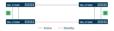
RSTP is designed for ease of use in multivendor environments. It is the most widely used and supported implementation of the spanning tree algorithm (STA) and is used in SEL network switches.
