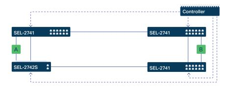
OT SDN is purpose-engineered for OT environments. SDN uses a secure control plane in which all primary and backup network paths are configured by a software flow controller. SEL devices support OT SDN.
