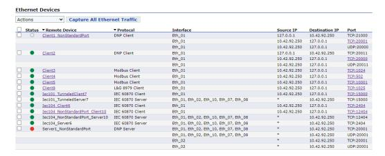
For SEL-3350, SEL-3555, and SEL-3560 RTACs, an online packet dissector is also available from the Connected IEDs page. This tool supports online trouble-shooting of device communications by providing real-time decoding of Ethernet and serial variations of devices of the following client/server protocols:
