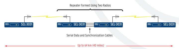
SEL-3031 Radios may be connected "back-to-back" to create a repeater. The repeater configuration can be used to extend the length of a link or to maintain radio contact when there is an obstacle between two sites.
