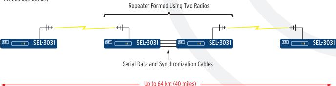
SEL-3031 Radios may be connected "back-to-back" to create a repeater. The repeater configuration can be used to extend the length of a link or to maintain radio contact when there is an obstacle between two sites.
