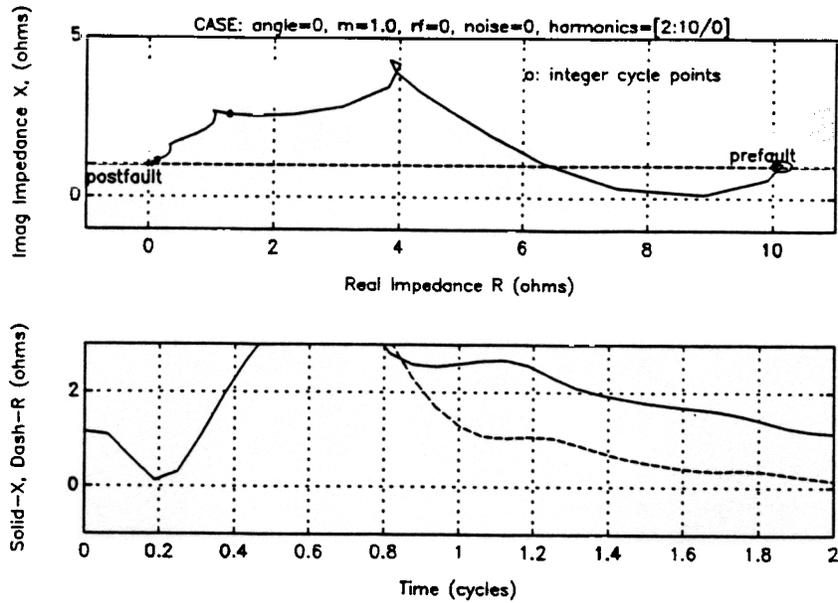
**Figure 4.6 Impedance Plot of Two-Cycle Cosine Filter**
