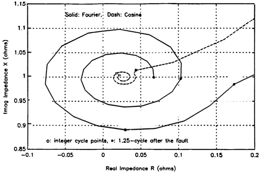
**Figure 6.5 Comparison of Cosine and Fourier Filters**
