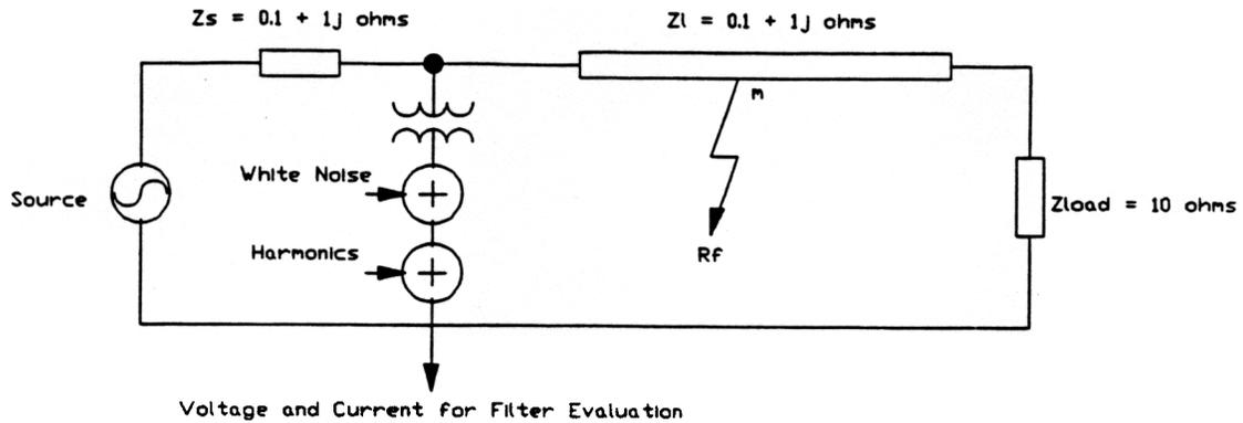
**Figure 5.1 Power System Model**
