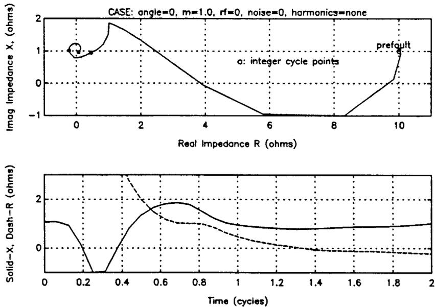
**Figure 6.7 Impedance Plot of the IIR Filter**
