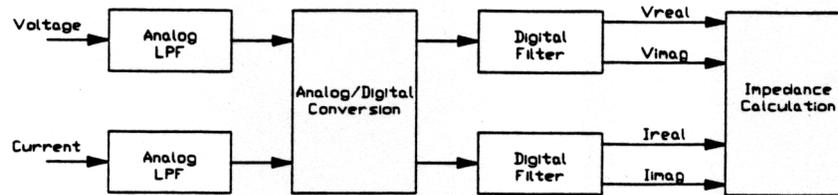
**Figure 5.3 System for Evaluating Analog and Digital Filters**
