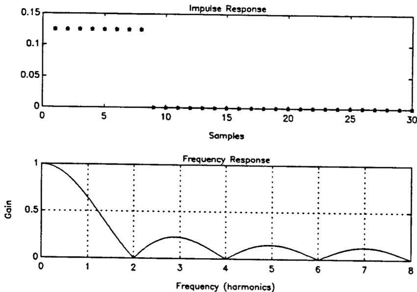
Figure 4.2 FIR Lowpass Filter  $y_k = [x_k + \dots + x_{k-7}]/8$
