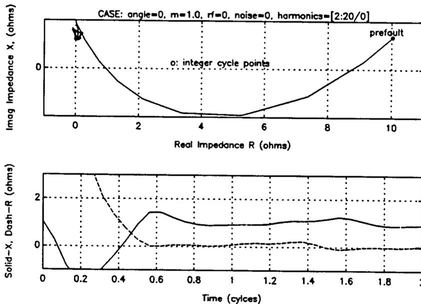
**Figure 6.11 Impedance Plot of IIR Correlator Filter**
