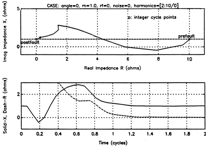
**Figure 4.5 Impedance Plot of One-Cycle Cosine Filter**
