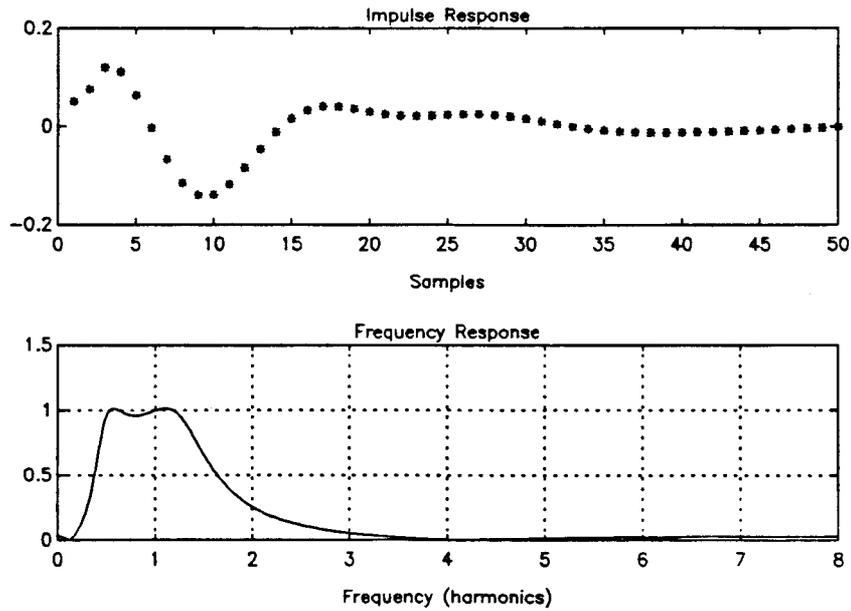
**Figure 6.6 An IIR Bandpass Filter**
