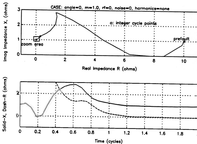
**Figure 6.3 Impedance Plot of Cosine Filter**
