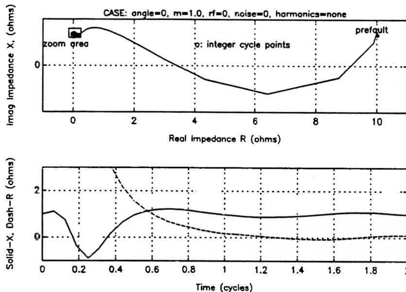
Figure 6.4 Impedance Plot of Fourier Filter
