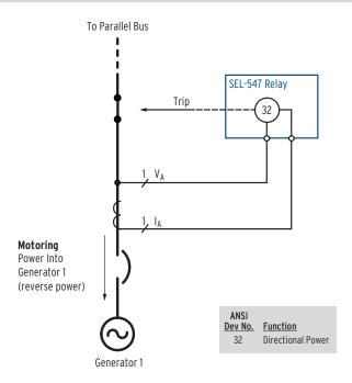
In the figure above, the generator normally operates in a parallel mode. For some reason (e.g., the generator loses its prime mover), power from the power system flows into the generator, motoring the generator. The directional power element in the SEL-547 detects this potentially damaging reverse power flow and trips the switch/breaker, breaking the parallel operation.
