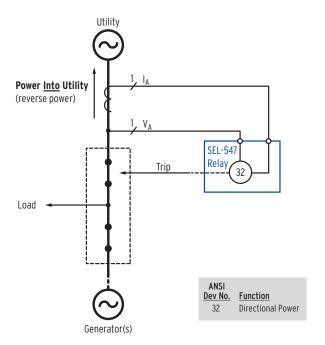
In the figure above, the generator normally operates in a parallel mode, but with the restriction that no power can be exported to the utility. Due to reduced onsite demand or some other phenomenon, a net flow of power into the utility results. The directional power element in the SEL-547 detects this reverse power flow and trips the transfer switch, separating the utility supply from the load and generator.
