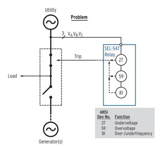
These two figures show the operation of the SEL-547 and an emergency backup generator for a system disturbance. The emergency backup generator is normally offline. In the first figure, the over-/undervoltage or over-/underfrequency elements in the SEL-547 detect local system islanding or a system-wide problem and trip the transfer switch, separating the utility supply from the load. A separate control (not shown) brings the emergency backup generator online, and the
