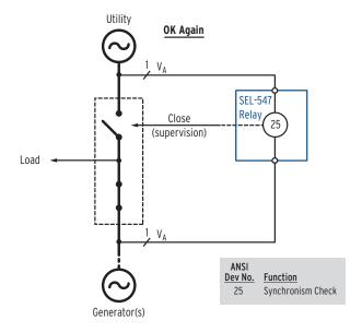
generator then supplies part or all of the load. Later, as shown in the second figure, the synchronism check element in the SEL-547 detects that the utility supply and generator are within normal bounds (voltage, frequency, and angle). The SEL-547 then issues a close (supervision) signal to a separate control (not shown) to close the transfer switch, reconnecting the utility supply to the load.
