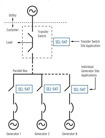
Apply the flexible SEL-547 at the transfer switch site (interconnection point between the utility and the customer) and at each individual generator site, as shown in the figure at left.
