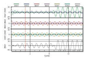
Use ACSELERATOR Analytic Assistant SEL-5601 Software to show quarter-cycle reports that include all analog and digital element values for digital evaluation of protection scheme performance.
