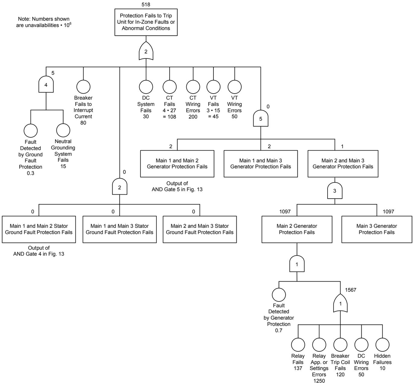
Fig. 14. Dependability fault tree for the two-out-of-three voting generator protection scheme.
