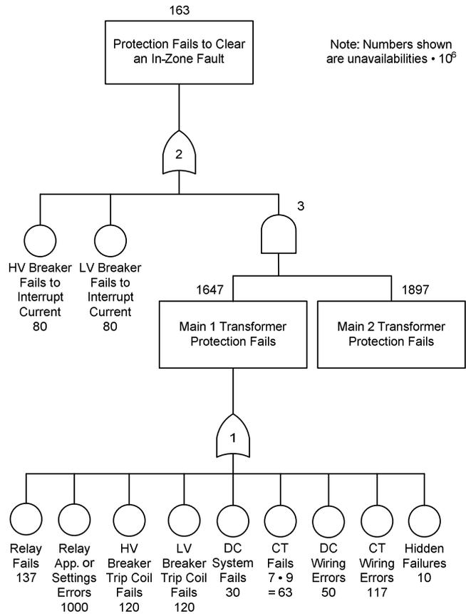
Fig. 5. Dependability fault tree for the dual-redundant transformer protection scheme, using relays from the same manufacturer.
