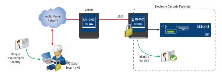
Use the PC Serial Security Kit to secure existing dial-up infrastructure, log and alert on access attempts, and authenticate to a remote security perimeter with a unique cryptographic identity.
